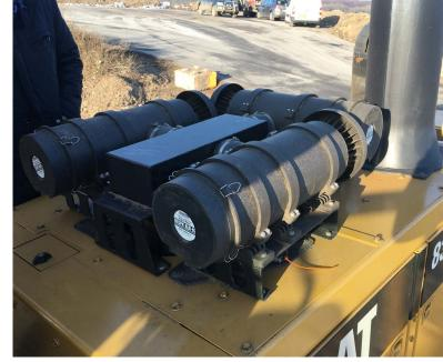
The XLR<sup>®</sup> covers engine air flows up to 9.9 m<sup>3</sup>/min with a single unit and much higher with muliple unit installations.
